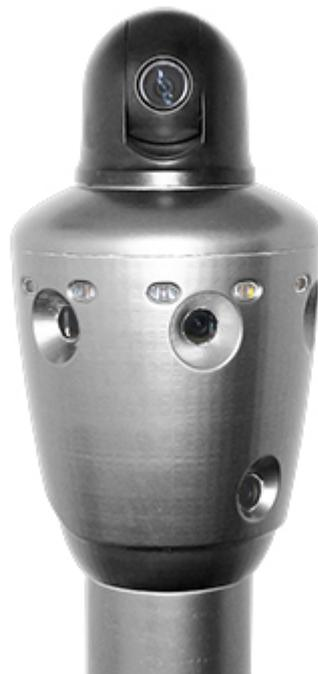
Security robot transmits highly informative picture of surrounding environment, taken by six cameras providing all-round video monitoring, and by one turning camera that automatically focuses on the source of movement. This configuration of video surveillance system allows getting a fully detailed picture of a suspicious moving object. Video surveillance system not only tracks moving objects and people, but also records captured video.
